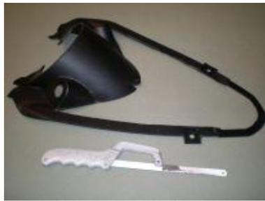
6. Attach the vent to the IP with the supplied rivets and back up washers. Washers go on the bottom to prevent the rivets from pulling through the plastic. You will require a drill with a 1/8" drill bit to make the holes.
